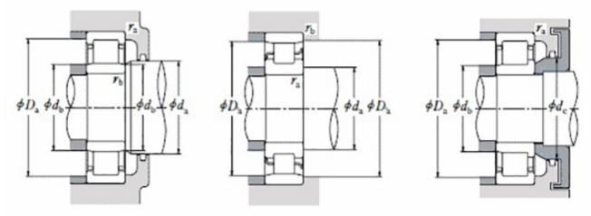
High quality cylindrical roller bearing with machined brass cage from the leading manufacturer TIMKEN. Featuring the TIMKEN EMA design. A premium land-riding cage, unique internal geometries, enhanced surface finishes and a compact design. All this adds up to longer life, improved uptime and reduced maintenance costs.
